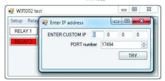
To test this you will need a computer that has its own internet connection and is NOT connected to the same network as the WIFI002. Download and run the <u>test program</u> above and select Custom IP. In the pop-up box enter your routers internet facing IP address. Click on "Try IP" and it will connect you to the WIFI002 just as if it were on your own network.
