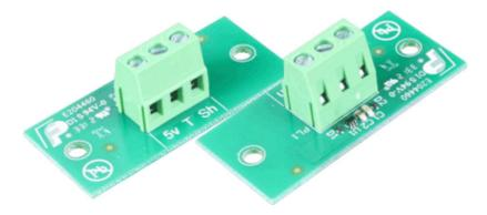
The TSA01 is a voltage output temperature sensor module employing Microchip's MCP9700A sensor.
