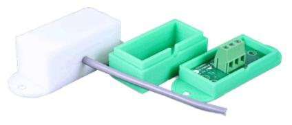
After wiring and testing the case is glued together and sealed.
