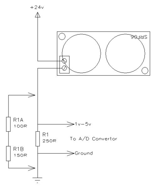
The SRF06 requires a minimum voltage of 9v. If 5v is being dropped across the 250 ohm resistor, then the minimum loop driving voltage is 14v (9v+5v).
