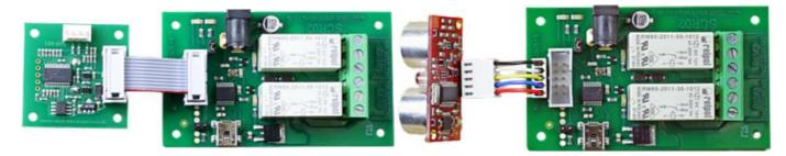
The photo's above illustrate the easy 1:1 connections between the SCR02 and our ultrasonic rangers. The SRF485 and SRF08 are used as examples, but any listed sonar connects as easily.
