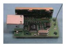
The RF04 is a very easy to use radio telemetry module. The module is powered from the USB bus, so no external power supply or batteries are required. Just plug it into your PC and it will appear as a COM port. The RF04 module can be used by anyone who can program a PC to use the COM ports.
