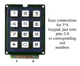
Pins 1 and 9 are unconnected - only pins 2 - 8 are used.
