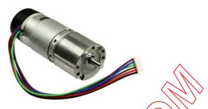
The EMG30 (encoder, motor, gearbox 30:1) is a 12v motor fully equipped with encoders and a 30:1 reduction gearbox. It is ideal for small or medium robotic applications, providing cost effective drive and feedback for the user. It also includes a standard noise suppression capacitor across the motor windings.
