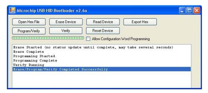
Now briefly press the reset button or click "Reset Device". This will reset the module and run your application.
