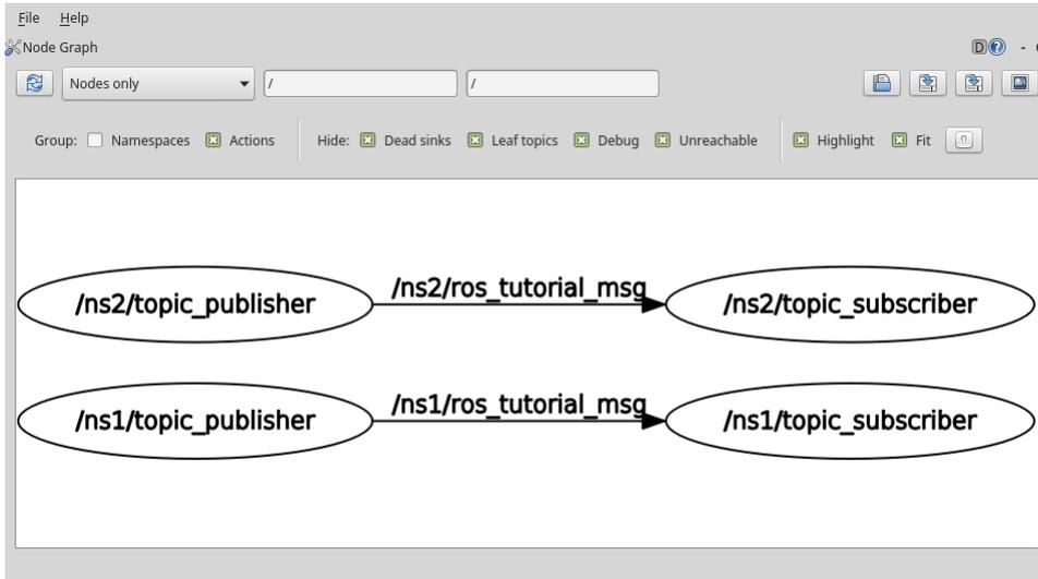
FIGURE 7-11 Message communication when using namespace
