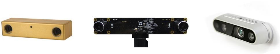
FIGURE 8-13 From left Bumblebee, OjOcamStereo, RealSense
