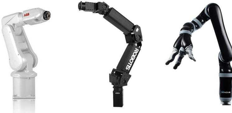
FIGURE 13-6 Various manipulators with ROS support (from left : ABB, ROBOTIS, Kinova)
