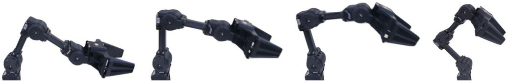
FIGURE 13-44 Operation of the OpenManipulator Chain
