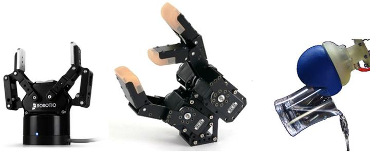
FIGURE 13-3 Types of grippers (from left: ROBOTIQ, ROBOTIS, Cornell University)
