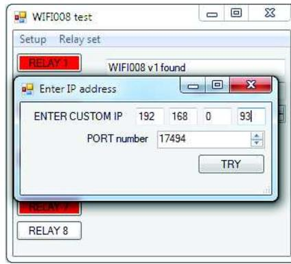
To test this you will need a computer that has its own internet connection and is NOT connected to the same network as the WIFI008. Download and run the [test program](#) above and select Custom IP. In the pop-up box enter your routers internet facing IP address. Click on "Try IP" and it will connect you to the WIFI008 just as if it were on your own network.
