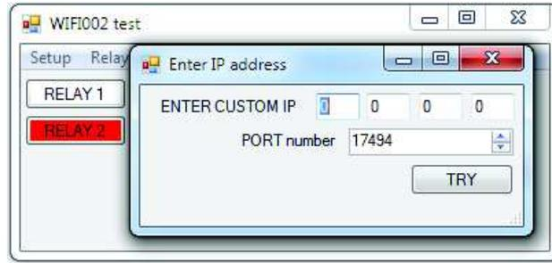
To test this you will need a computer that has its own internet connection and is NOT connected to the same network as the WiFi002. Download and run the [test program](#) above and select Custom IP. In the pop-up box enter your routers internet facing IP address. Click on "Try IP" and it will connect you to the WiFi002 just as if it were on your own network.
