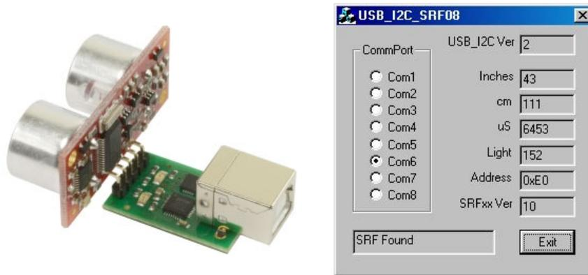
The connector on the USB-I2C module may be soldered directly to the SRF08 as shown, or you can use a cable if preferred. The USB-I2C module can easily supply the 25mA peak of the SRF08. The software automatically searches for the SRF08 and displays its I2C address, along with revision number, range and light sensor reading. You can download [usb\\_i2c\\_srf08.exe](#) and the [C source code](#) here.
