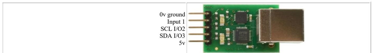
The diagram below shows the I2C connections.
