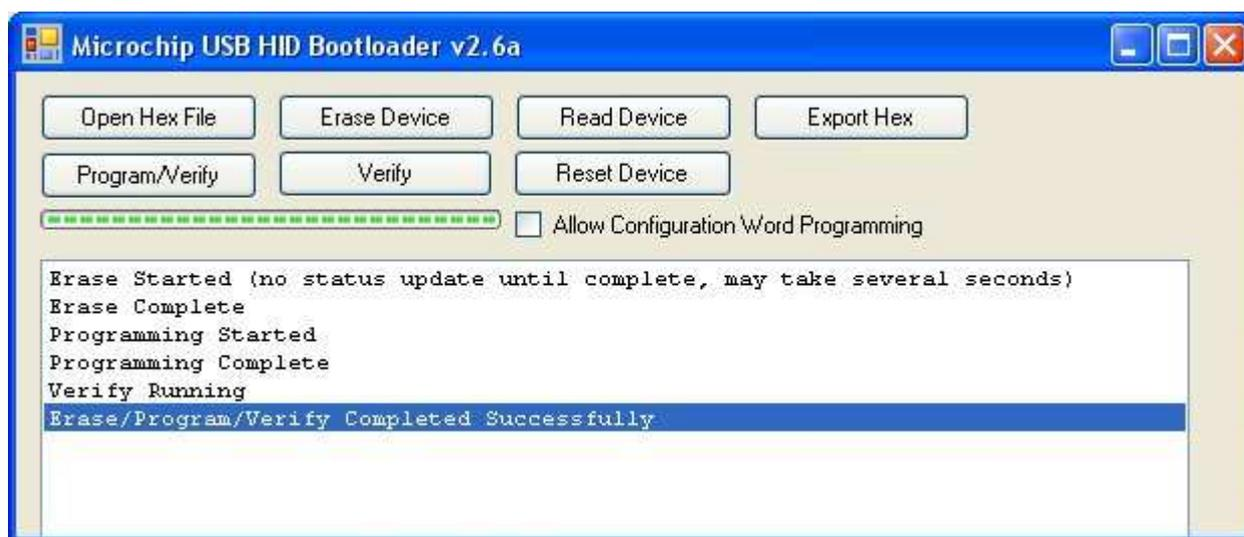
Now remove the link between pin1 and 0v ground and press "Reset Device". This will reset the module and run your application.
