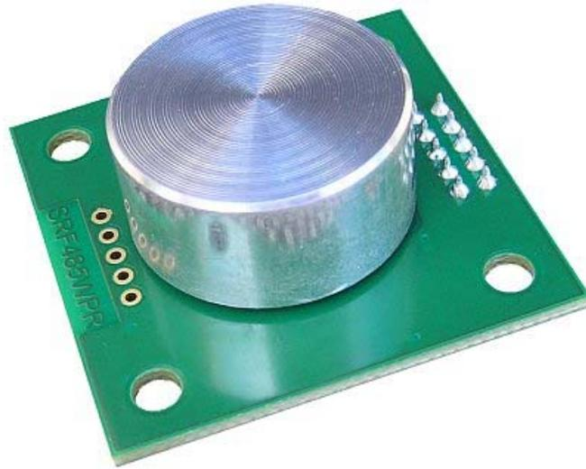
**Note - This sonar has a waterproof transducer, not an underwater transducer. It is designed for operation in air.**
