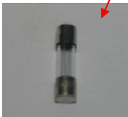
(3) Separate the burnt fuse from the CM-5 circuit board.
