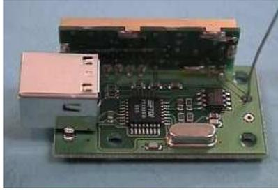
The RF04 is a very easy to use radio telemetry module. The module is powered from the USB bus, so no external power supply or batteries are required. Just plug it into your PC and it will appear as a COM port. The RF04 module can be used by anyone who can program a PC to use the COM ports.
