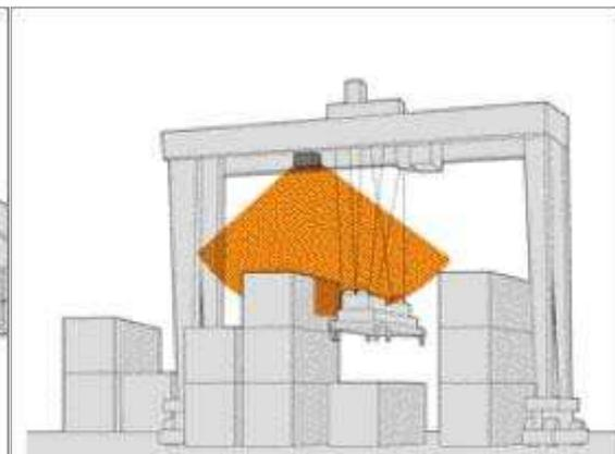
Area monitoring for collision prevention of RTGs, RMGs and AGVs
