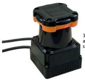
30m scanning range. Suitable for security purpose as a monitor in outdoor environment. also possible for sticking-out detection.
