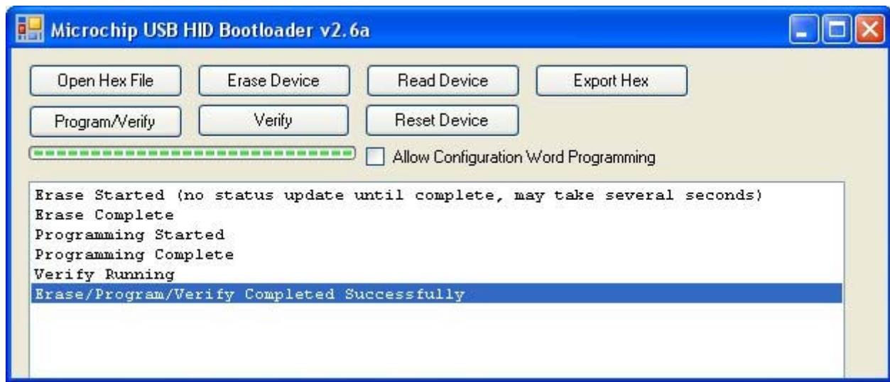
Now briefly press the reset button or click "Reset Device". This will reset the module and run your application.
