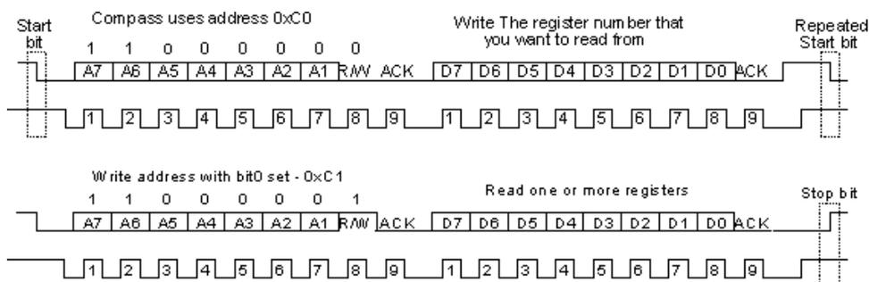
First send a start bit, the module address (0XC0) with the read/write bit low, then the register number you wish to read. This is followed by a repeated start and the module address again with the read/write bit high (0XC1). You now read one or two bytes for 8bit or 16bit registers respectively. 16bit registers are read high byte first. The compass has a 16 byte array of registers, some of which double up as 16 bit registers as follows;
