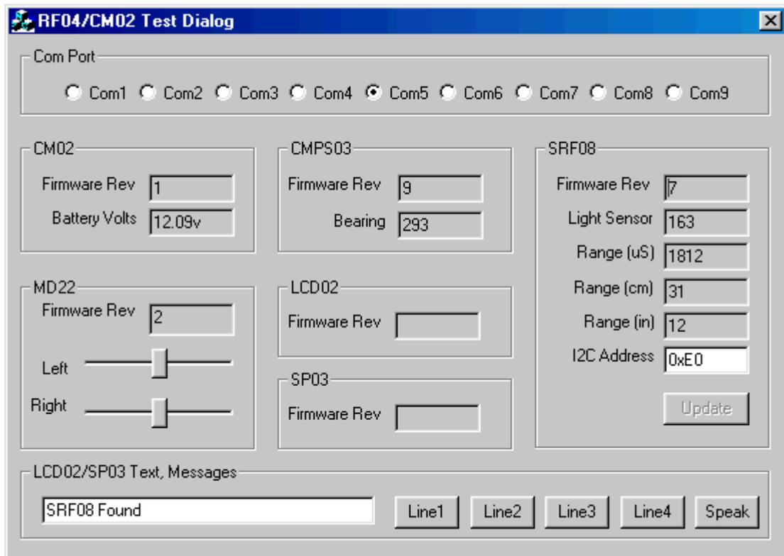
In this case Rev1 and 12.09v coming from the battery. In this example the CM02 is fitted to our test robot - Chucky. It has an MD22 fitted to drive the motors, and you will see this is firmware Rev2. The sliders controls the speed of the motors. There is a CMPS03 compass module fitted - Rev9 and showing a bearing of 293 degrees. An SRF08 has been found at address 0xE0. Chucky actually has 12 SRF08's fitted, the one shown is simply the first
