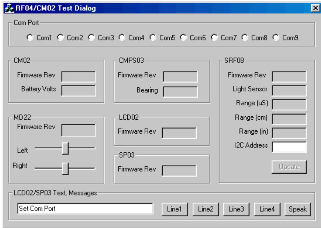
You should first select the com port that the RF04 has been instantiated to. There are instructions on the [RF04 technical page](#) about how to find which com port its located at. You only have to set the com port once. If you have a CM02 powered up and in range, you will see the Firmware Revision and Battery voltage appear on screen.
